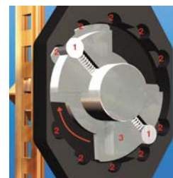
During the turn movement, the safety pins ① are moved along the swivel clutch ③ into further recesses ② where they again audibly engage.
